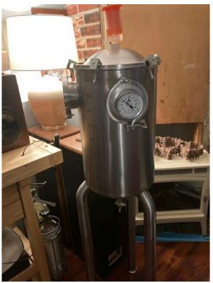
Before using it as a fermenter, I pressurized it with compressed air. It held pressure but only under 5 PSI.
